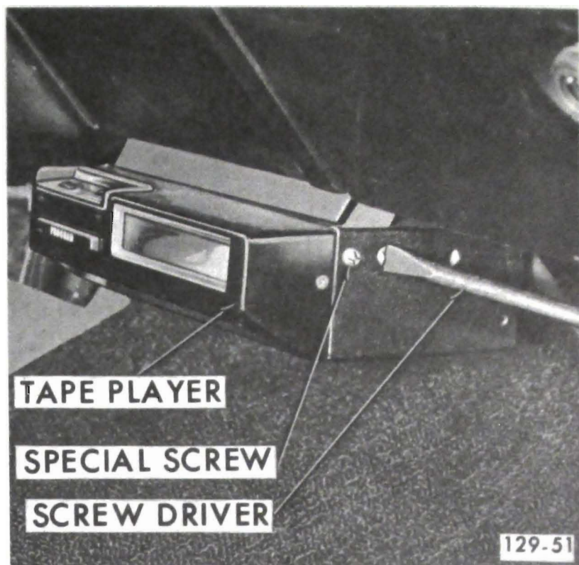
Figure 129-16 Anti-Theft Screw Removal
