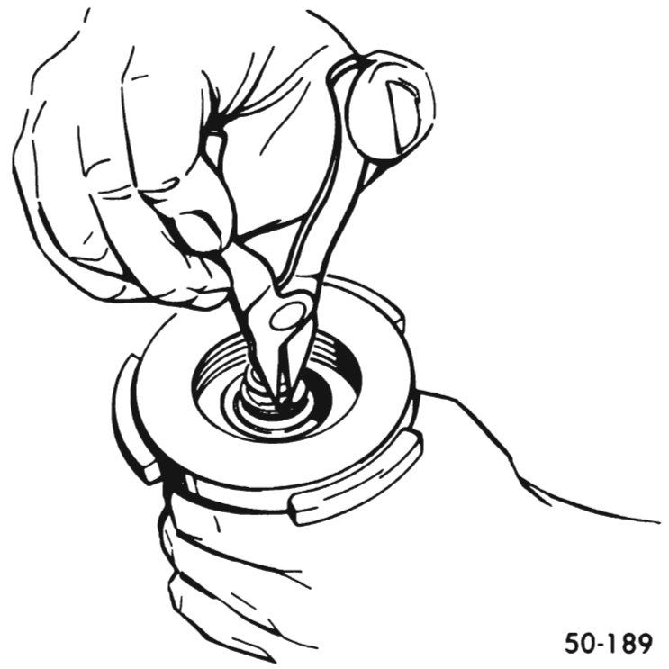
Figure 50-82 Removing Retaining Ring From Air Valve
