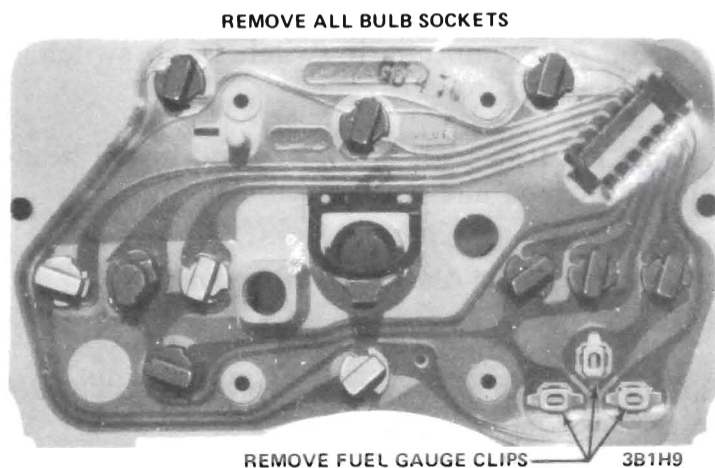
Figure 1H-9 Removing Printed Circuit
