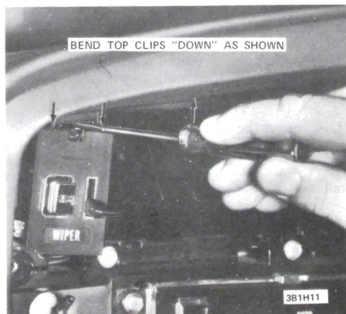
Figure 1H-11 Releasing Top of Switch Assembly
