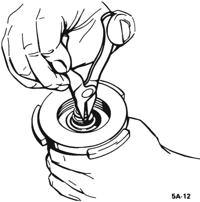
Figure 5A-12 Removing Retaining Ring From Air Valve
