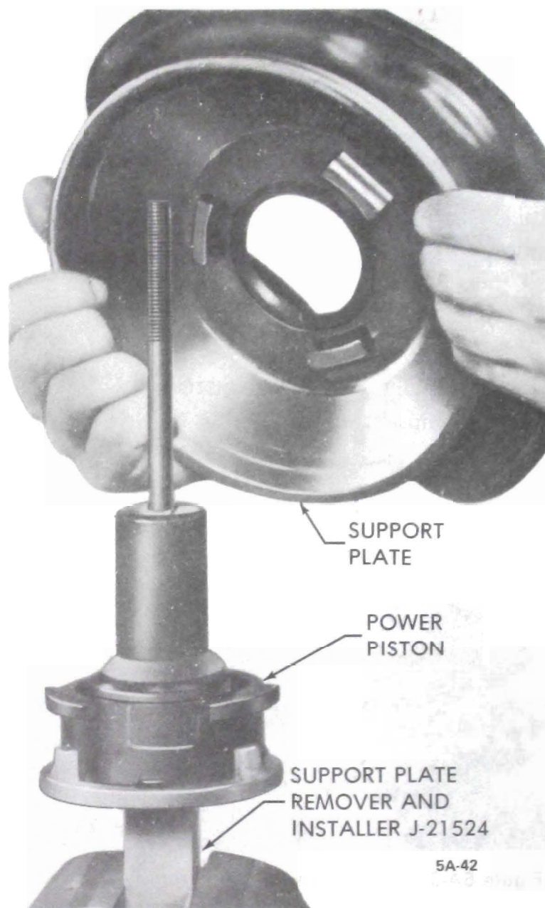
Figure 5A-42 Removing Support Plate
