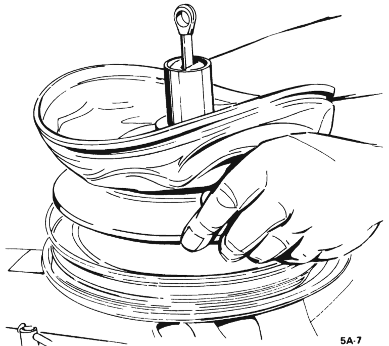
Figure 5A-7 Locking or Unlocking Primary and Secondary Power Pistons
