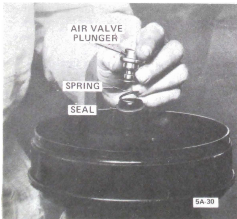
Figure 5A-30 Installing Air Valve Plunger
