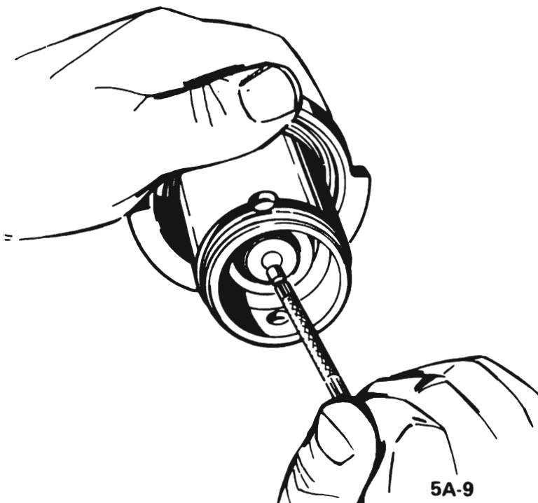
Figure 5A-9 Removing Reaction Piston and Reaction Disc From Secondary Power Piston
