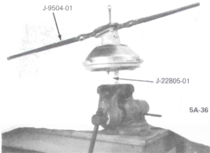
Figure 5A-36 Separating Power Brake Unit
