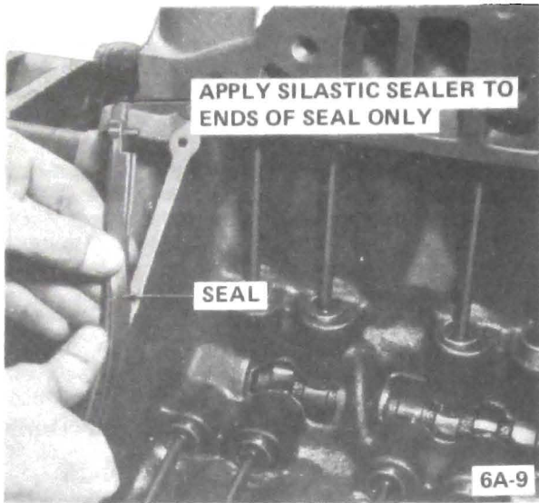
Figure 6A-9 - Intake Manifold Seal Installation
