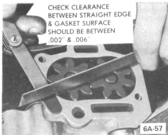
Figure 6A-57 - Checking Oil Pump End Clearance
