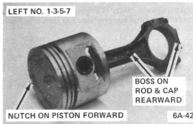
Figure 6A-42 Left Bank Piston and Rod Assembly (350 Cu. In. with Cap crew Rods)
