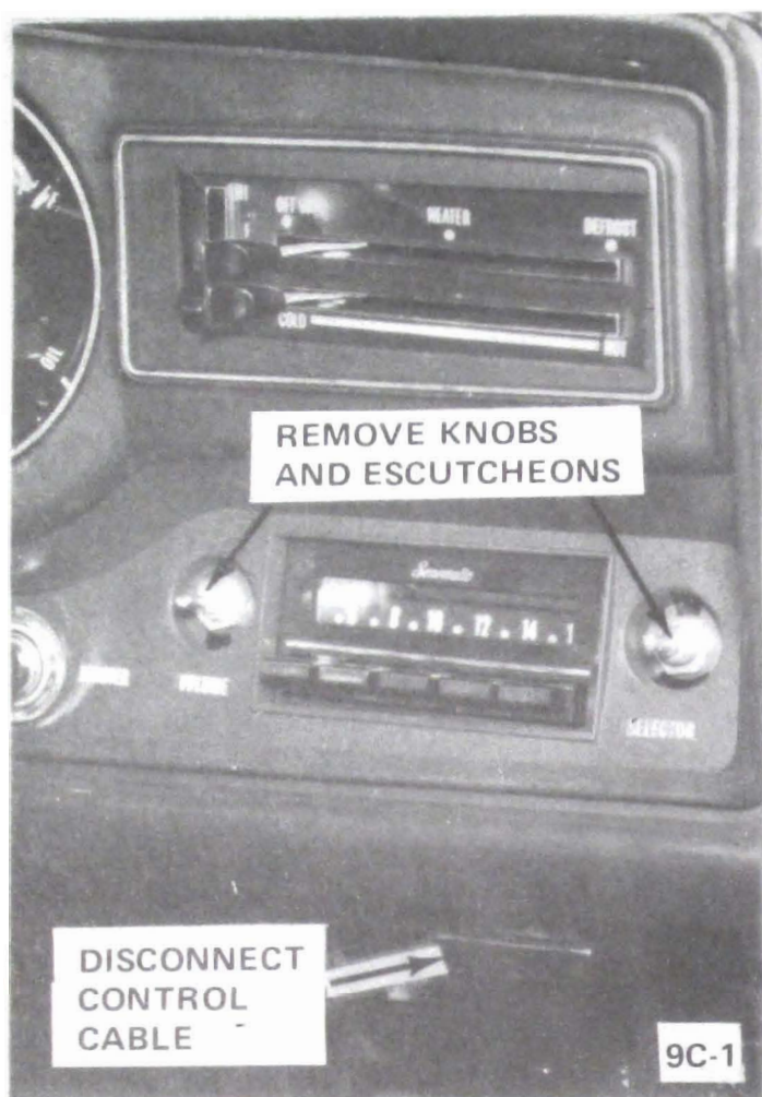
Figure 9C-1 Center Air Duct Control
