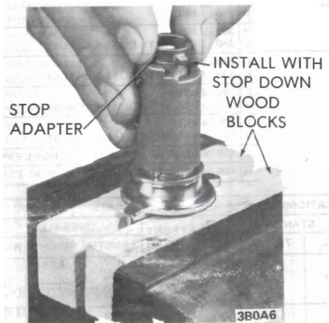
Figure 0A-6 Installing Stop Adapter on Lock Cylinder
