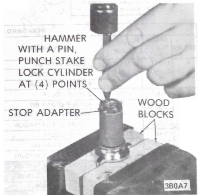
Figure 0A-7 Staking Lock Cylinder to Retain Lock Adapter
