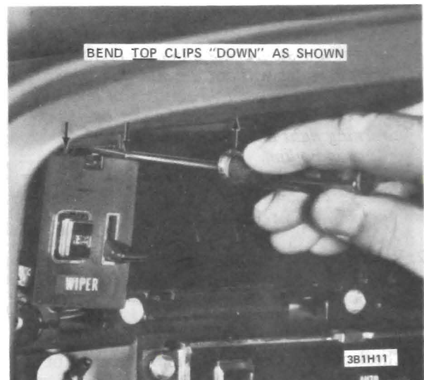
Figure 1H-11 Releasing Top of Switch Assembly
