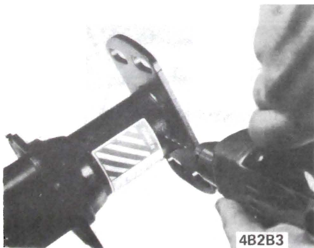
Figure 2B-3 Relieving Pressure Before Scrapping
