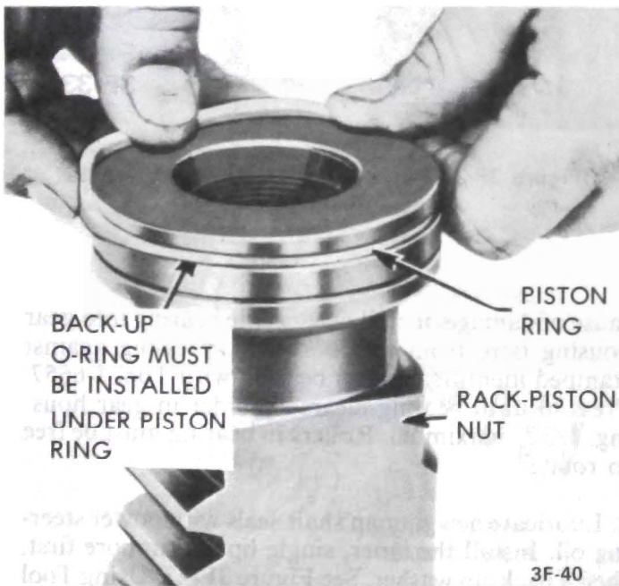
Figure 3F-21 - Installing Ring on Rack Piston
