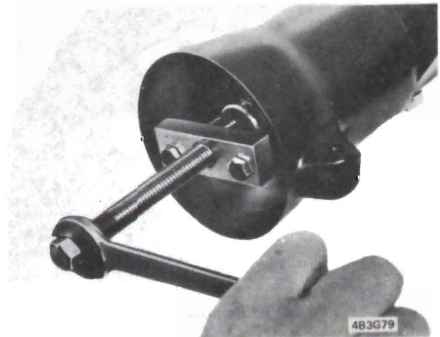
Figure 3G-79 Removing Shift Tube
