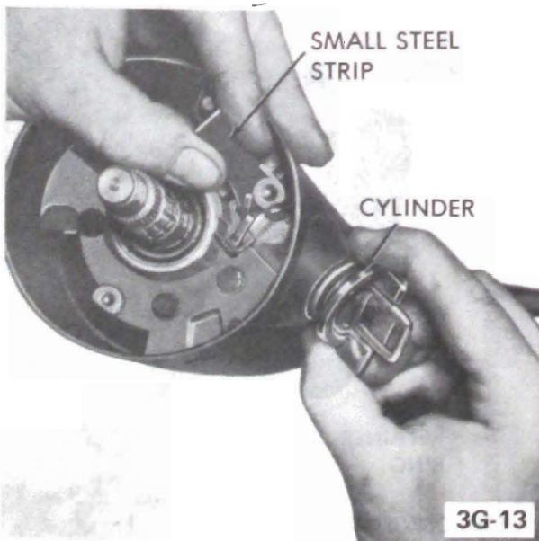
Figure 3G-33 Removing Ignition Lock Cylinder
