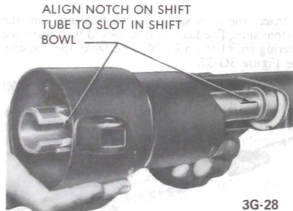
Figure 3G-48 - Installing Shift Bowl
