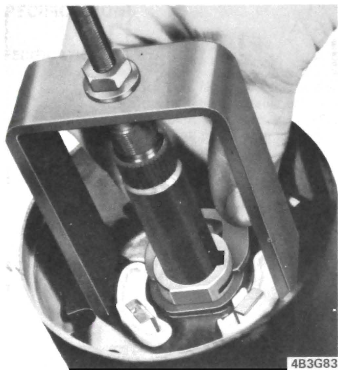
Figure 3G-83 Installing "C" Ring
