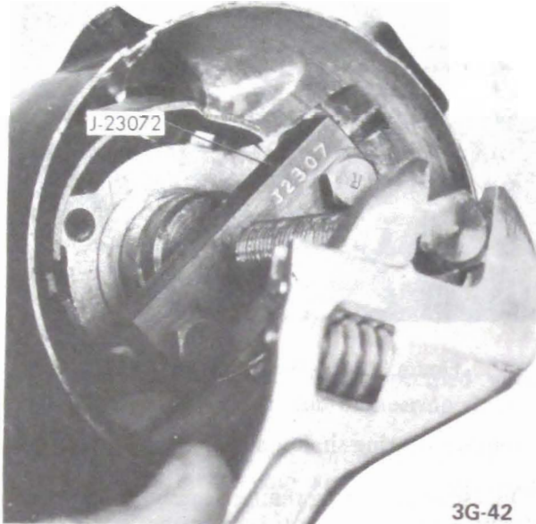
Figure 3G-62 - Removing Shift Tube
