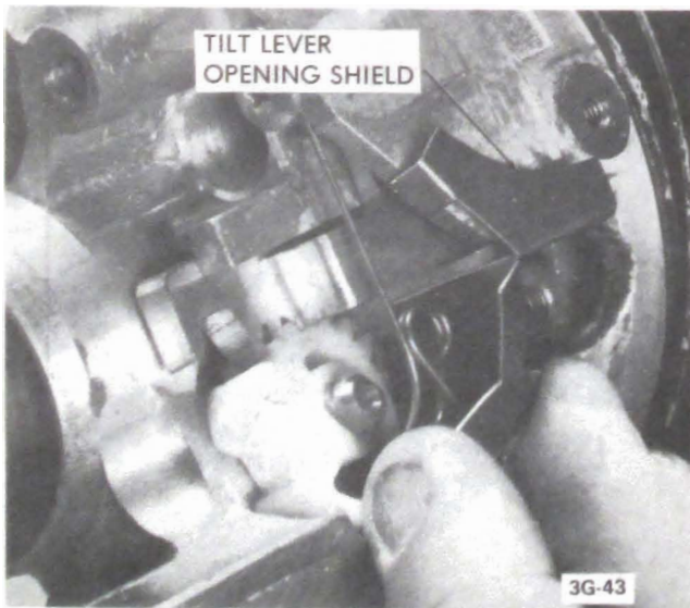
Figure 3G-63 - Removing Tilt Lever Opening Shield
