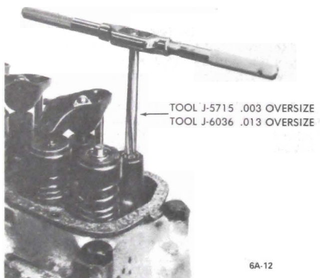
Figure 6A-12 Reaming Rocker Arm Stud Hole
