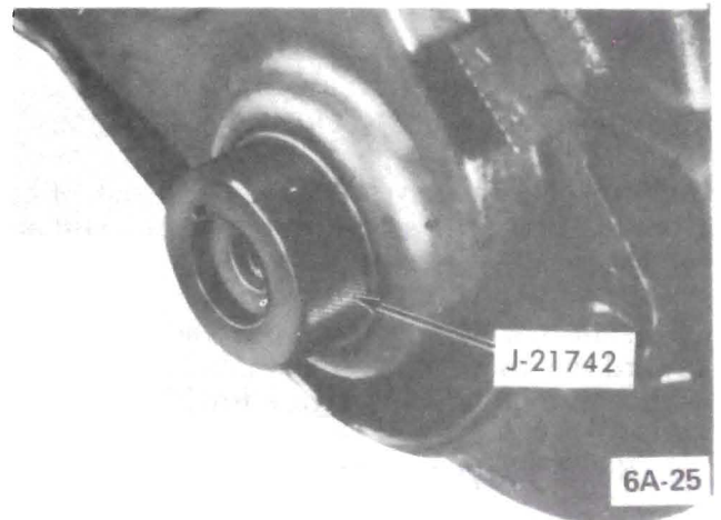
Figure 6A-25 Installing Centering Tool in Cover
