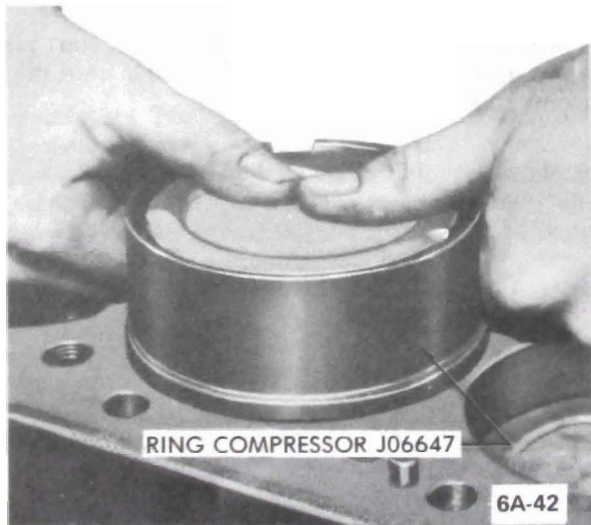
Figure 6A-42 Installing Piston with Ring Compressor
