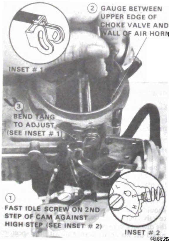
Figure 6E-25 - Fast Idle Cam Adjustment
